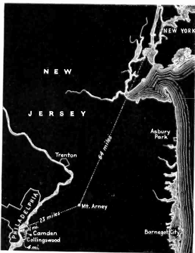
Path of 49-50 megacycle waves from New York to Camden which underwent one radio relay enroute to be rebroadcast and "seen" at Collingswood
