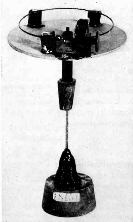
Photographs of two resonators used by Heinrich Hertz in his demonstration of the existence of electric waves
